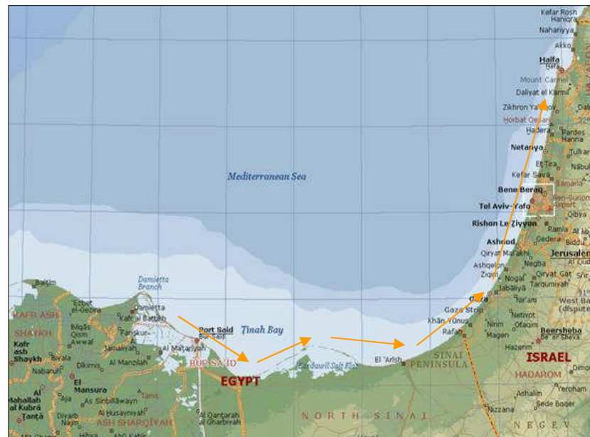
Fig. 1. Nile littoral cell location map (arrows indicate net longshore sediment transport direction)
