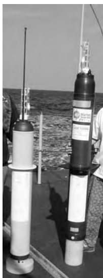
Fig. 5. Argo profiling floats (Apex to the left and Provor to the right) ready to be deployed in the Eastern Mediterranean.
