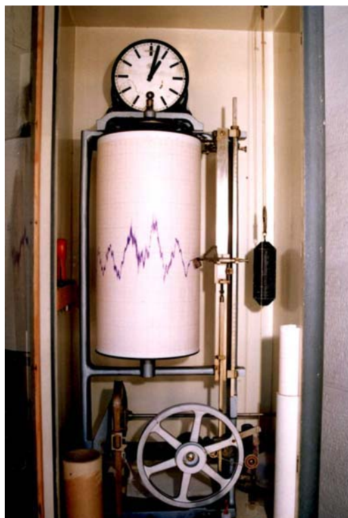
Fig. 2 Mechanical tide-gauge A. Ott – Kempten at Split.
