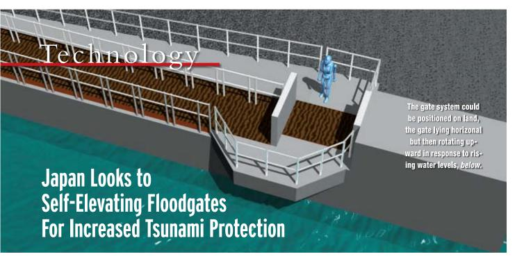
COASTAL BARRIER system that is being developed in Japan elevates automatically in response to unusually high water levels and holds promise for protecting people and property from such disasters as the one that struck the northeastern part of the country in early 2011. The so-called flap-gate tsunami breakwater system would operate without electric power, rising into position through its natural buoyancy in the event of unduly high tides, floods, or tsunamis.
